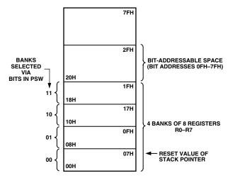
Figure 2. Lower 128 Bytes of Internal RAM
